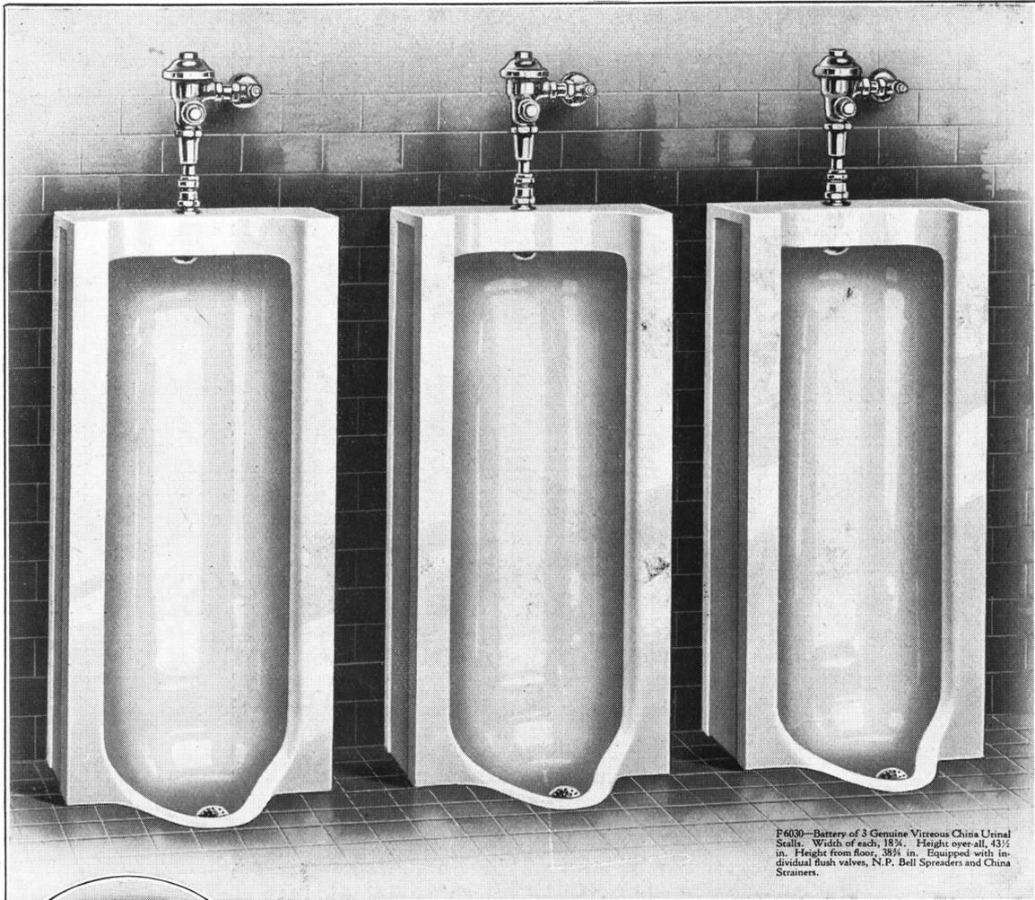
F6030—Battery of 3 Genuine Vitreous China Urinal Stalls. Width of each, 18 3/4". Height over-all, 43 1/2" in. Height from floor, 38 3/4" in. Equipped with individual flush valves, N.P. Bell Spreaders and China Strainers.
